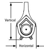
Horizontal Clearance Required Standard Duty: 110 mm (4-1/4") Heavy Duty: 135 mm (5-1/4")
